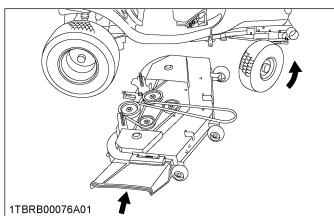
4. Attach the mower deck to the link and mower link with 2 clevis pins and 4 rue-ring pins.
