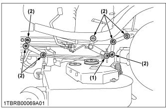
Around the pin (1) (2) Pivot of mower link
