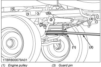
Engine pulley (1) (2)Mower belt
