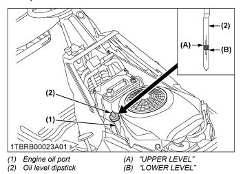
3. To check the oil level. Remove the dipstick, wipe it clean, insert it and draw it out again. Check to see that the oil level is between the 2 marks.
