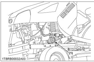
(1) Engine oil filter cartridge
