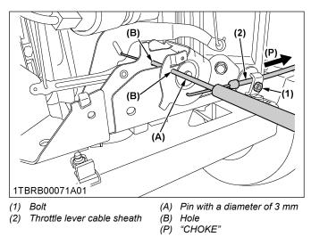
3. If not possible, loosen the bolt (1) and pull the throttle lever cable sheath (2) in the direction of the arrow so that the pin (A) passes through all the required holes (B). And then tighten the bolt (1).
