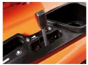
Hydraulic mower lift lever
