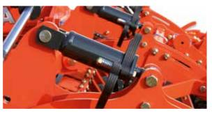
The working depth can easily be adjusted by pivoting spacers, no matter if it is manually (only on mounted models) or hydraulically.
