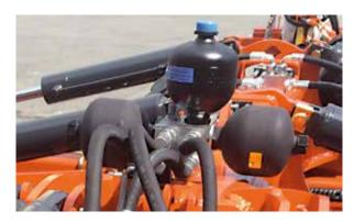
The CD1000T and CD2000T are extremely stable as they are equipped with a double suspension device that protects the frame against stress and increase tremendously the stability of the machine during work.
