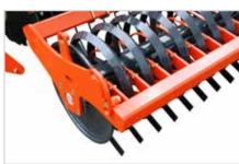
Actiring ø 540mm - 160 kg/m The Actiring roller using the same frame structure and knife system than the Actipack but discs are replaced by a "V" profile ring. This saves 60kg/m, which is of critical importance for reducing lifting capacity. Actiring is not recommended in stony conditions.
