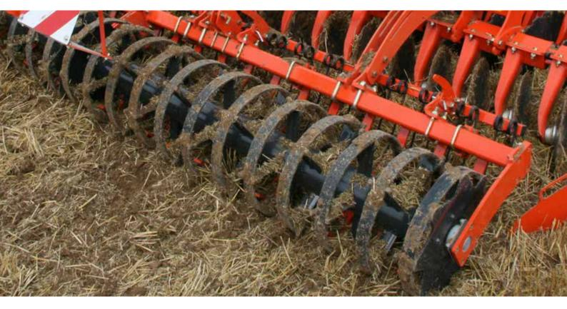
Consolidation is an elementary action of arable farming. Reducing large open pores and aggregate size allows for improved seed-to-soil contact and keeping the water necessary for the next crop germination. The right choice of the right roller depends on the soil type and conditions. Also, lifting capacity of the tractor needs to be considered. Therefore, Kubota offers a wide range of maintenance-free rollers to finalise the levelling and re-consolidation of the soil.
