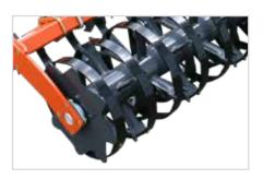
Actiflex ø 580mm - 160 kg/m The Actiflex roller has been made to create an intensive mixing and create a nice seedbed with all soil types, even stony conditions. The rings made with spring steel are separated by skids to have a high resistance against stress at high speed and enhance weeds regrowth after harvesting.
