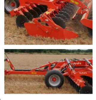
The adjustable lateral side deflectors on the right and left-hand side control the soil flow to provide a perfect level finish. All discs are working at the same depth, even the outer ones. The lateral deflectors are parallelogram mounted which allows them to follow the ground contours and control the soil flow at the same time.
